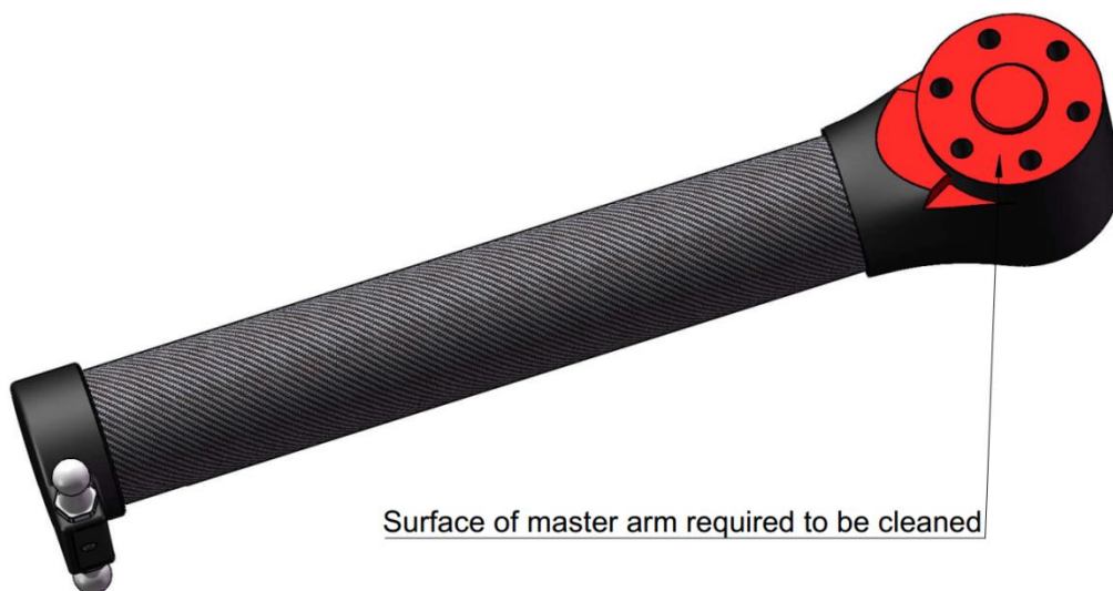
Figure 3-9 Schematic diagram of master arm mounting surface
